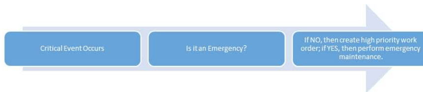
Fig 13.2: Work Flow of Emergency Maintenance
